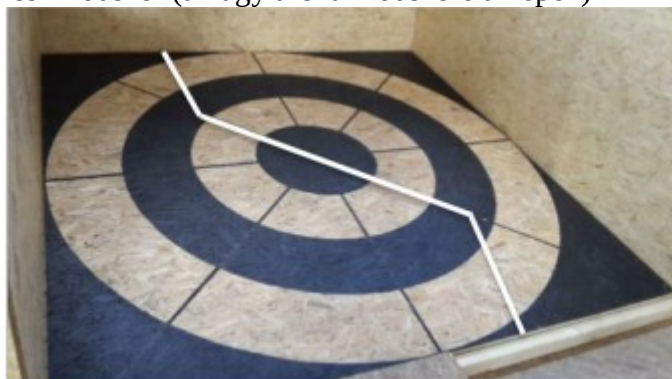
Figure 6: Traverse Testing Method (Major Arena Method Pictured)
