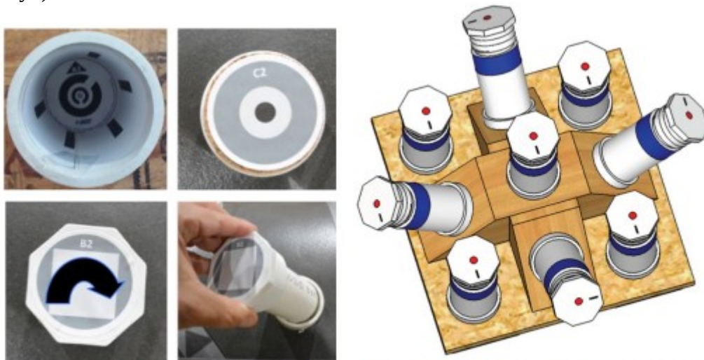
Figure 12: (L) The four dexterity tests: Inspect, Precision touch, Rotate and Extract. (R) The nine locations on a dexterity board where the test is to be performed.
