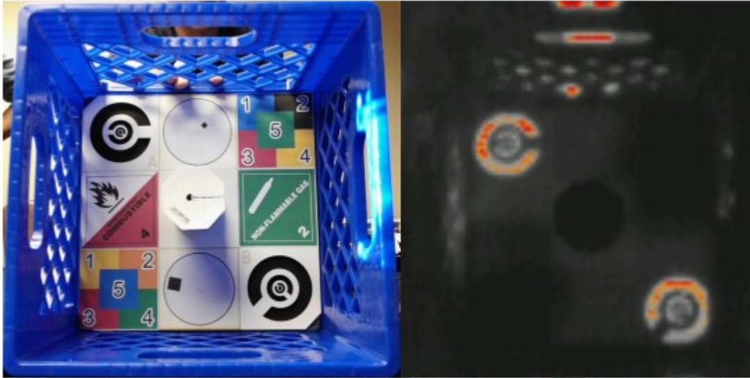
Figure 14: Crate with sensor tests, clockwise from top left: Visual/Thermal Acuity, Motion, Colour, Hazmat, Visual/Thermal Acuity, Motion, Colour, Hazmat. Note that the dexterity manipulation object in the centre is ignored for RMRC as dexterity manipulation is evaluated elsewhere. Audio acuity (a speaker playing a computer-generated voice speaking numbers and letters) and CO2 are not visible in this picture.
